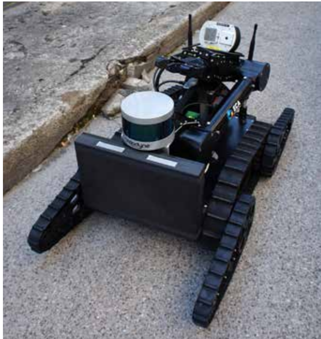
◀ The NERVA XX robot from Nexter Robotics with the miniaturised gamma camera from CEA and the FPG detector from Arktis Radiation Detectors mounted.
