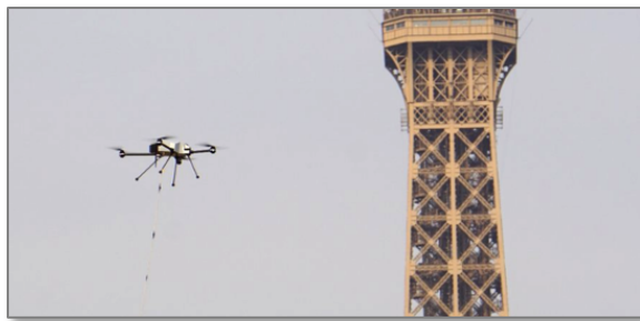
The Q800X UAV can be deployed tethered (left) or autonomously (right) with the “dronebox”, enabling 24/7 autonomous take-off/landing and battery recharging. Image copyright © Aeraccess
