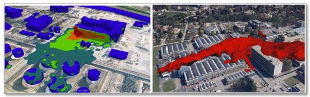
The 3D computer model of the radiation plume (top) is dynamically updated with the measurement data from UAV/UGV. The contamination information is provided via 4G or WIFI to operators using augmented reality (below), compatible with the Bruhn NewTech Frontline application, used in the monitoring and management of CBRN events. Image copyrights: Top 2 images © École Centrale de Lyon. Lower image © Luxembourg Institute of Science and Technology.
